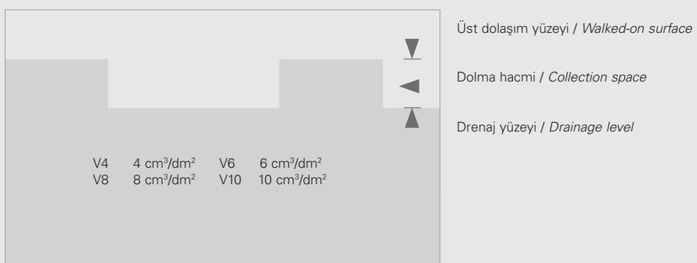
Karo kesiti / Cross-section of tile
